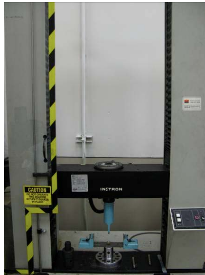
Figure 37 Instron Testing Machine with 3 Point Flex Test Fixture
