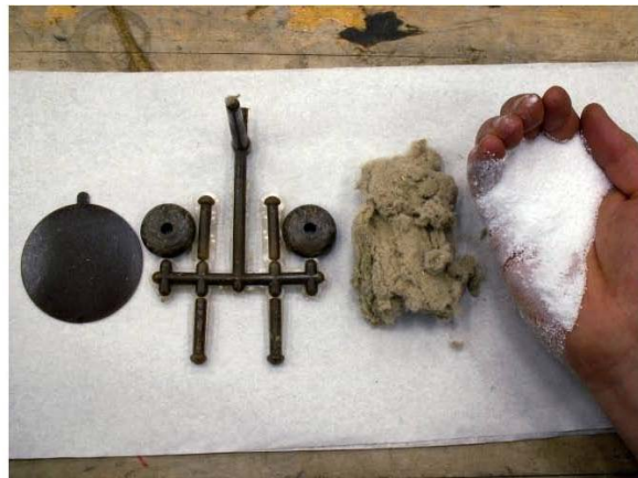
Figure 32 From right - neat resin in hand; flax fibers; hand mixed and injection molded sample; pelletized and injection molded
